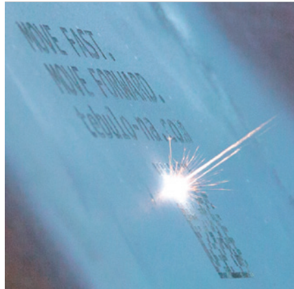
LASER ETCHED MARKING
