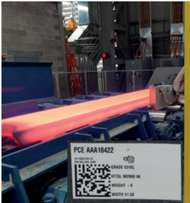
HOT SLAB TAGGING
